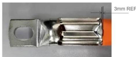
Figure 7: Crimp the ring tongue
