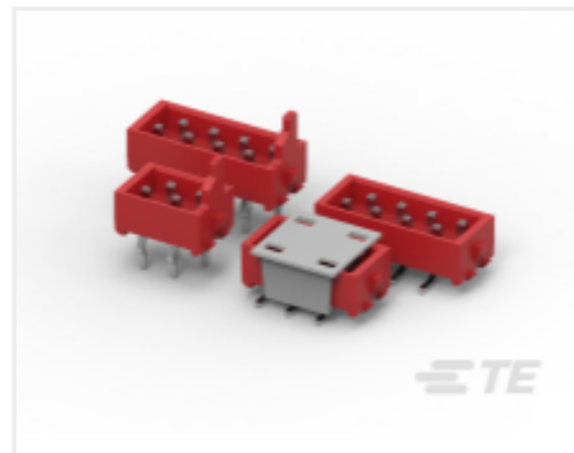
TE Part #7-215464-4 Male-on-Board Connector, Micro-MaTch
