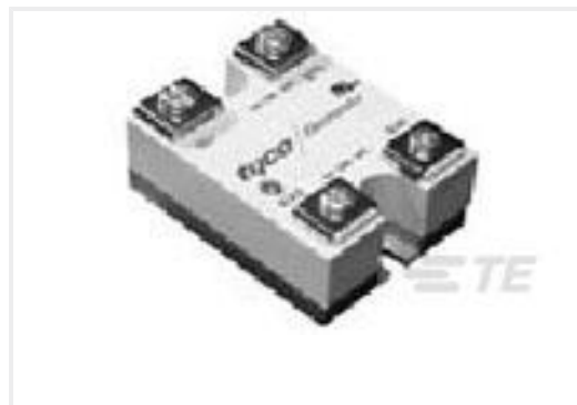
TE Part #1393030-4 SSR-240A25= PANEL MOUNT,25A, 240VAC-AC i/p
