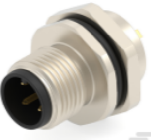
TE Part #T4132012041-000 M12,FRONT MOUNT,MALE,A,4P, SOLDER WIRE
