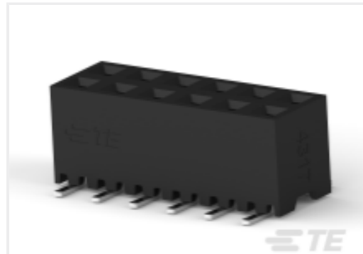
TE Part #1-2314846-2 12P,2MM,BB,REC,DRVT,SMD,AU.76, TB,W/CP
