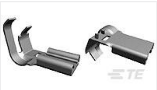
TE Part #1742543-1 250 FASTON,FLAG,REC.,18-12 AWG, NPST
