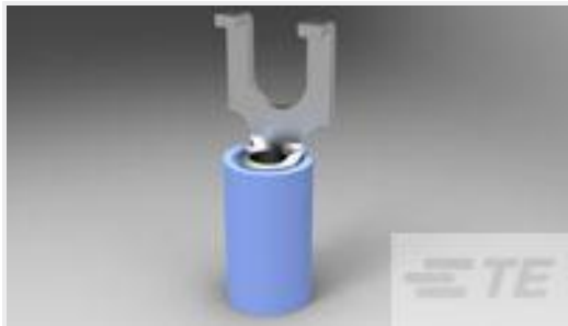
TE Part #8-320862-1 TERMINAL,PIDG SPD FLG 16-14 8
