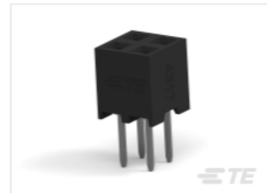
TE Part # 2307786-4 4P,2MM,B-B,REC,DRVT,2.7,0.76AU
