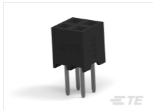
TE Part # 2307785-4 4P,2MM,B-B,REC,DRVT,2.0,0.76AU
