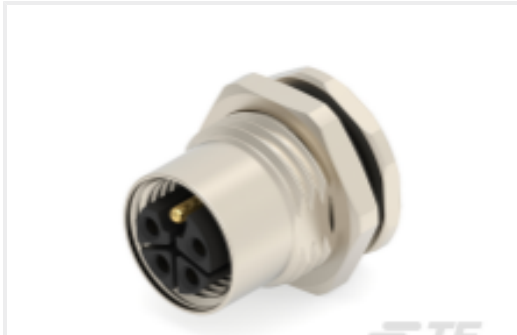
TE Part #T4141L12051-000 M12,REAR MOUNT,FEMALE,L,4P+PE, SOLDER PCB
