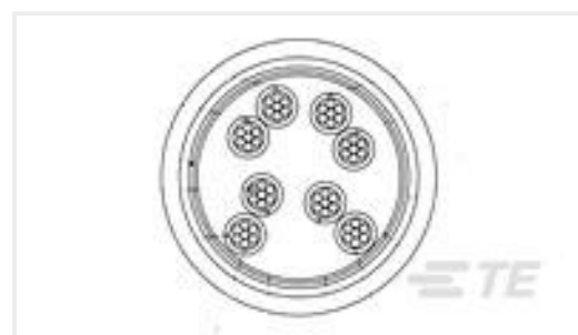
TE Part #1939708-1 Industrial Ethernet Cat5e (AWG)
