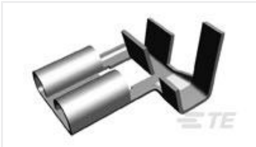
TE Part #63963-1 250 FASTON FLAG REC 18-14 AWG NPST
