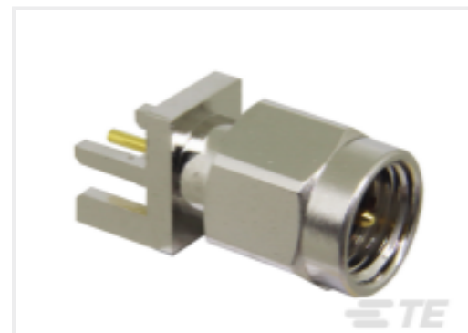
TE Part #L9000275-01 SMA Plug 50 Ohm .062 PCB Edge Mount
