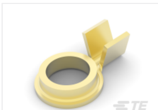
TE Part #160088-3 RING TONGUE 20-16 AWG 0.198 X . 700 BR
