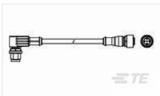
TE Part #1-2273122-2 M12 angled plug to M12 strgt socket AA
