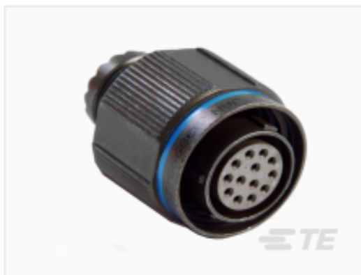
TE Part #YDTS26F13-35PNV001 Straight Plug: D38999, 13-35 Insert, Electroless Nickel Plating
