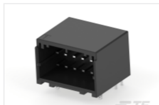
TE Part #2-1827875-3 Header Assembly: Wire-to-Board, 5A, gold or tin plated
