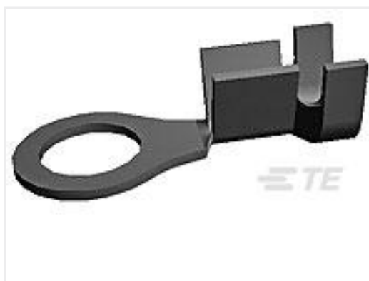
TE Part #40660 RING 164(4.17 MM) TERMINAL 18-14 AWG BR
