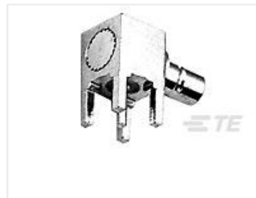
TE Part #1-1337481-0 SMB R/A PCB Skt 50Ohm Gold Plt
