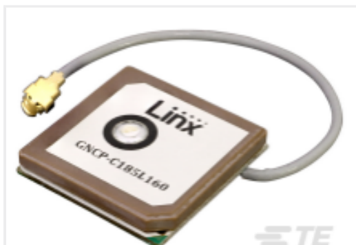
TE Part #ANT-GNCP-C185L160 Antenna GNSS L1 18x18 LNA 1.13 UFL
