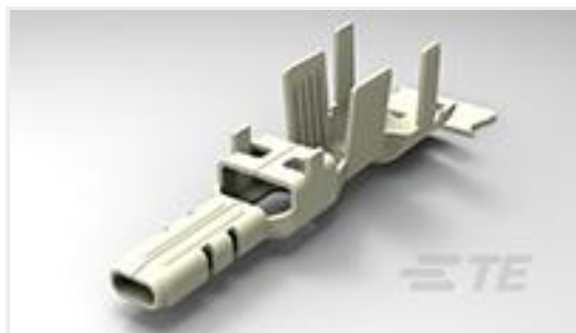
TE Part #1971786-1 PTL TAB CONTACT, 20 - 24 AWG
