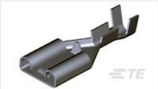
TE Part #63854-2 250 PL MKIII REC. 18-14AWG TPBR
