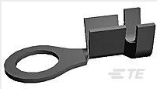
TE Part #160101-2 RING TONGUE 20-16 AWG 0.0253 TPBR
