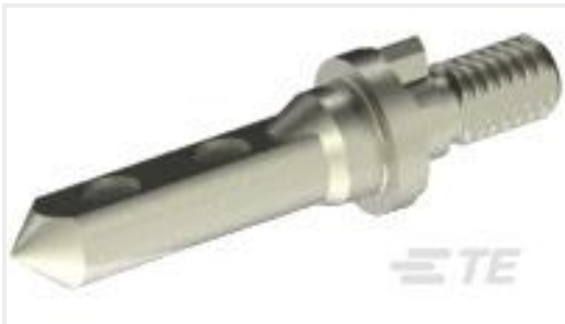
TE Part #1-1469491-2 MULTIGIG RT GUIDEPIN, 9MM 2.60
