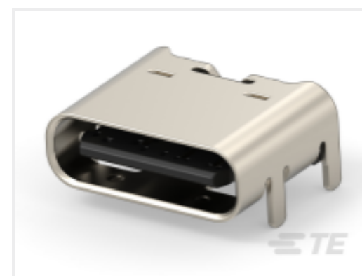
TE Part #2479774-2 USB C Charge-only, 6 Pin, Top, 3u GF
