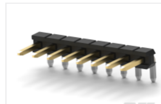
TE Part #1-2823104-0 10P,2MM,BRK HDR,SRRT,2.8,0.76AU, TB
