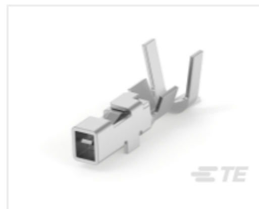
TE Part #1827588-2 Contact: Component To Wire; 3-5A, 30-18 Wire Size
