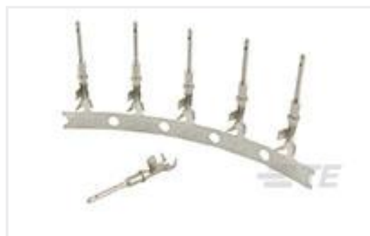
TE Part #1060-20-0122 PIN, SF, SIZE 20, 16-22, NI/NI
