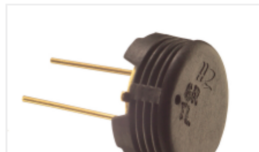
TE Part #HPP801A031 HS1101LF HUMIDITY SENSOR
