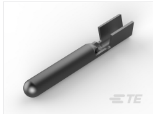
TE Part # 61013-2 PIN .109 (2.77 MM) 18-14 AWG TPBR
