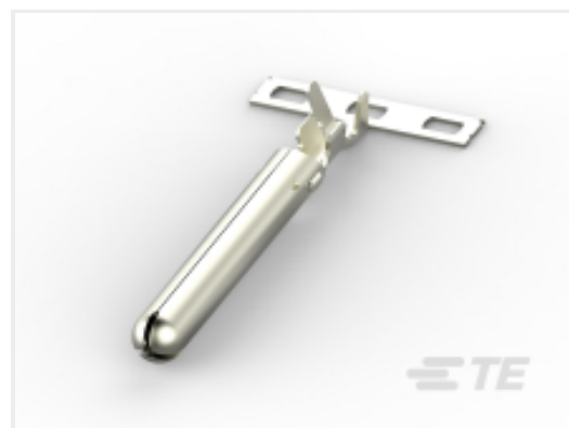
TE Part # 626361-3 WALL PLUG PIN 0.5/1.5MM2 0.38X36.40 NIBR
