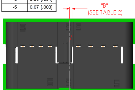
FINAL X AXIS LINEAR MISALIGNMENT
